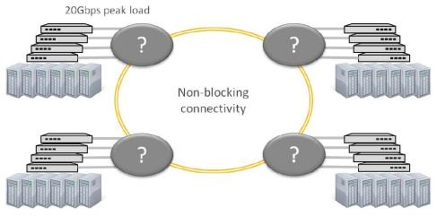
Fig. 4 Single data center spread across four locations
