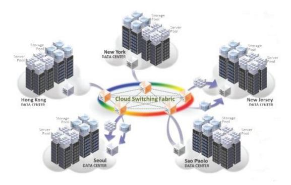
Fig. 2 VM and storage mobility across cloud data centers in a SDN networking environment
