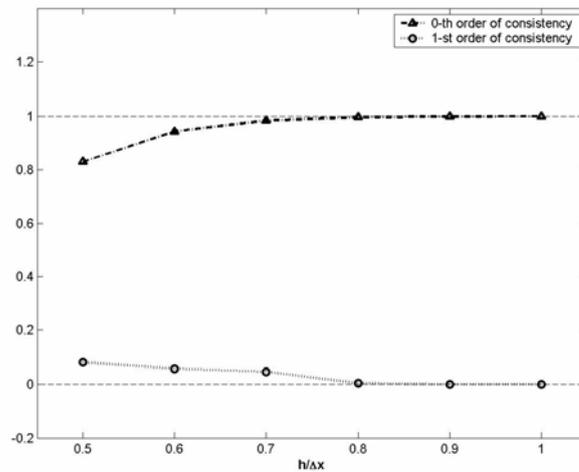
**Fig. 2** Set of  $b$  values by using conditions (7) for the Gaussian smoothing kernel function in 1-D.
