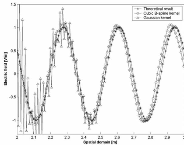
**Fig. 6** Comparison among the space profiles of theoretical propagating pulse and SPH simulations using the cubic  $B$ -spline and the Gaussian smoothing kernel functions with  $h=1.2\cdot\Delta x$ .
