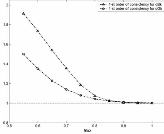
**Fig. 3** Set of  $b$  values for derivatives of the cubic  $B$ -spline (dBk) and the Gaussian (dGk) smoothing kernel functions in one-dimension.
