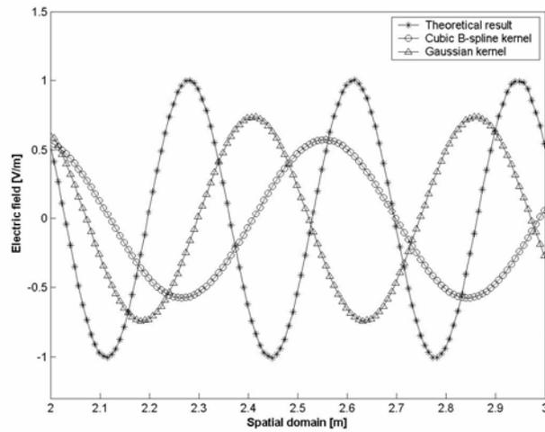
**Fig. 5** Comparison among the space profiles of theoretical propagating pulse and SPH simulations using the cubic  $B$ -spline and the Gaussian smoothing kernel functions with  $h=0.6\cdot\Delta x$ .
