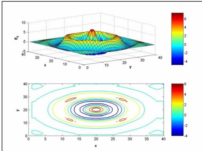
Fig. 11 Computed result with the cubic  $B$ -spline smoothing kernel function for the electric field  $E_z$ .
