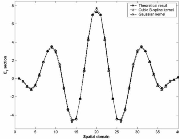
**Fig. 9** Section of space profiles of the electric field  $E_z$  at time step  $t=20$ .
