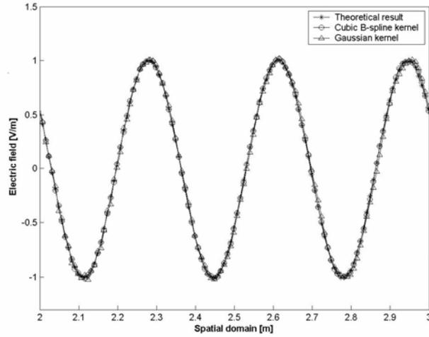
**Fig. 4** Comparison among the space profiles of theoretical propagating pulse and SPH simulations using the cubic  $B$ -spline and the Gaussian smoothing kernel functions with  $h=0.92\cdot\Delta x$ .
